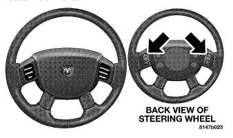
The right-hand control is a rocker type switch with a pushbutton in the center. Pressing the top of the switch will increase the volume and pressing the bottom of the switch will decrease the volume.
